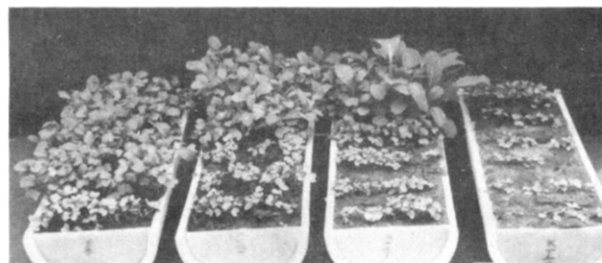
Figure 3. Mustard bioassay showing the distribution of chlorsulfuron in split soil leaching columns of the four soil types. From left to right: Acredale silt loam, Cullen clay loam, Roanoke sandy loam and Kenansville loamy sand. Front is the top of the column while the far end is the bottom.
